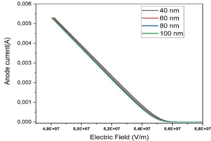
**Figure 9** Variation of the Anode Current as a Function of the electric Field for Different Thicknesses of the Active Layer
