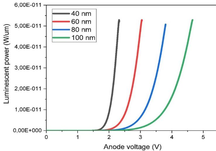
**Figure 8** Effect of Emitting Layer Thickness on Luminescent Power as a Function of Anode Voltage
