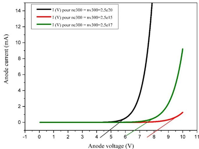
**Figure 10** Variations of I-V characteristics of OLEDs as a Function of Charge Carrier Density
