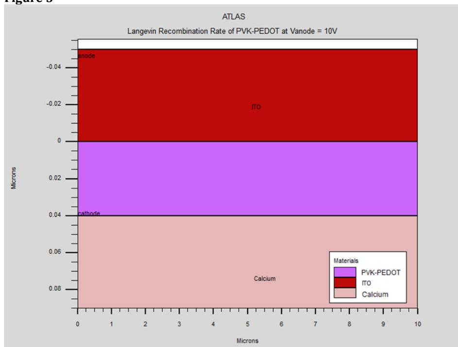
**Figure 5** Simulating OLED Structure using Silvaco Atlas
