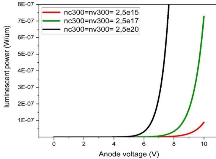
**Figure 11** Effect of Charge Carrier Density on Luminescent Power as a Function of Anode Voltage
