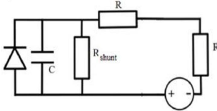
Figure 4 Structure of OLED
