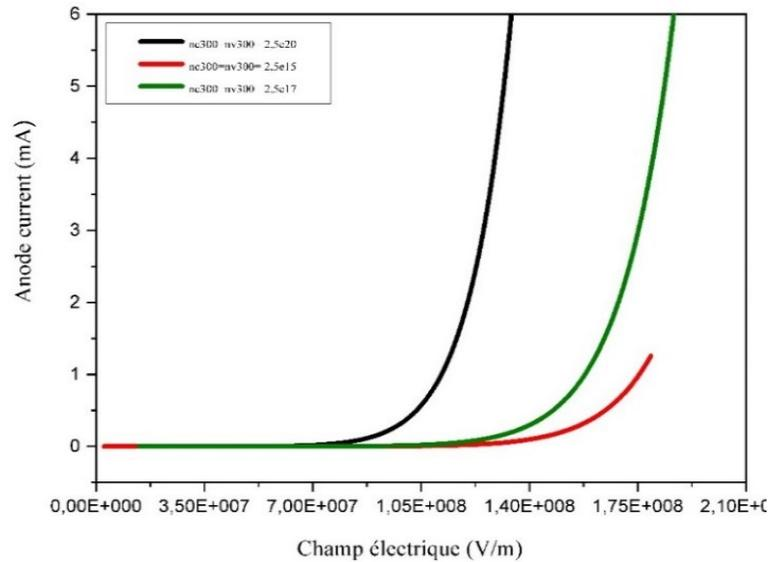
**Figure 12** Variation of the Anode Current as a Function of The Electric Field for Different Charge Carrier Density
