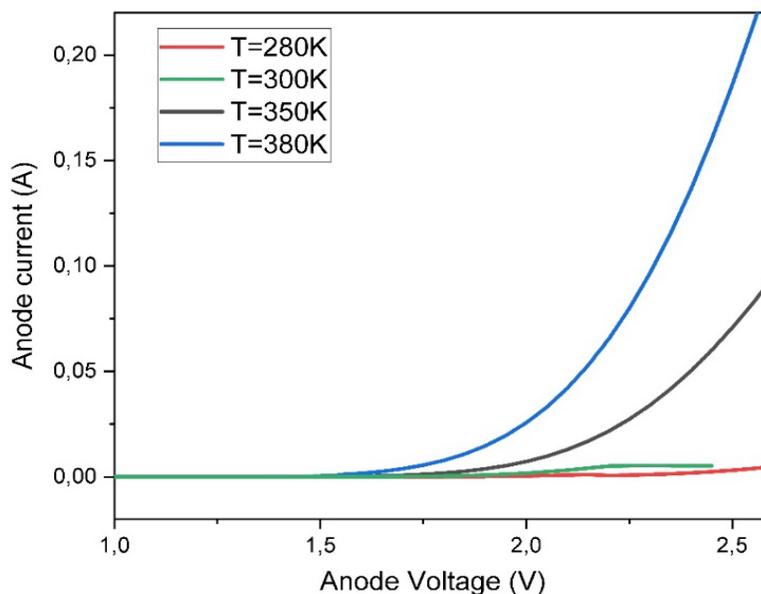
**Figure 13** Variations of I-V Characteristics of OLEDs as a Function of Temperature
