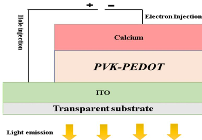
Figure 3 OLED Electrical Circuitry
