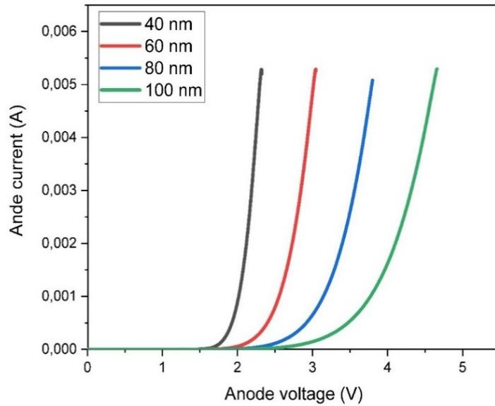
**Figure 7** Variations of I-V Characteristics of OLEDs as a Function of Emitting Layer Thickness.
