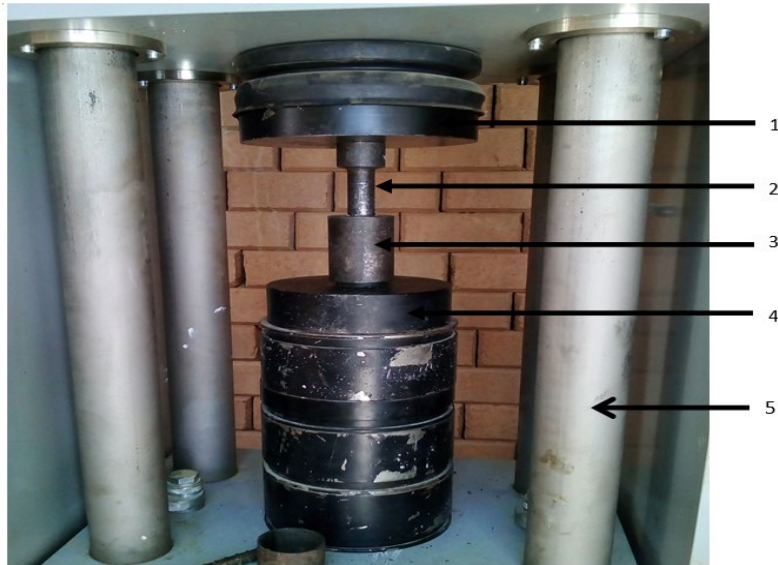
Plate 1 UT CO821 Compression Machine and Extrusion Setup (1-Machine Punch Head, 2-Rig Plunger, 3-Rig Cylinder, 4-Base Plate, 5-Machine Ram Travel Rail)
