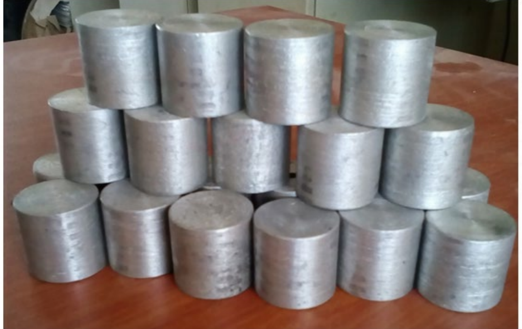
Appendix A 4 Aluminium Alloy Billets Machined to : \varnothing 25.3\text{mm} \times 25.4\text{mm}
