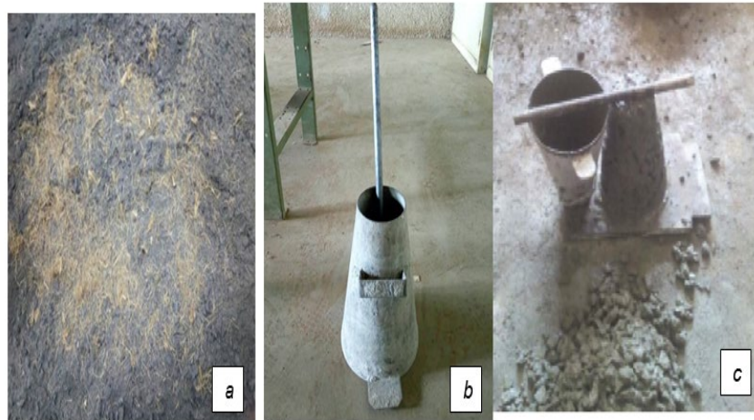
Figure 6 (a) Dry samples, (b) Slump cone (c) Samples from the cone
