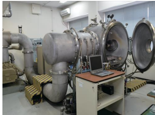
Figure 2: Erosion testing machine of JUTEM
