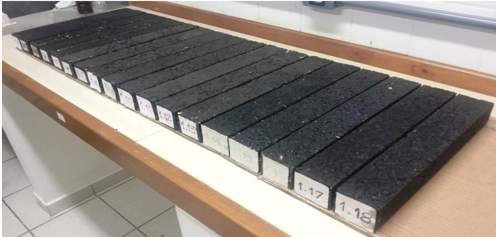
Figure 3: Prismatic specimens (beams) tested in this study.
