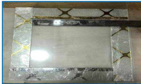
Figure 5: The casting mold consists of glass plates with dimensions (200 x 200 x 4 mm).
