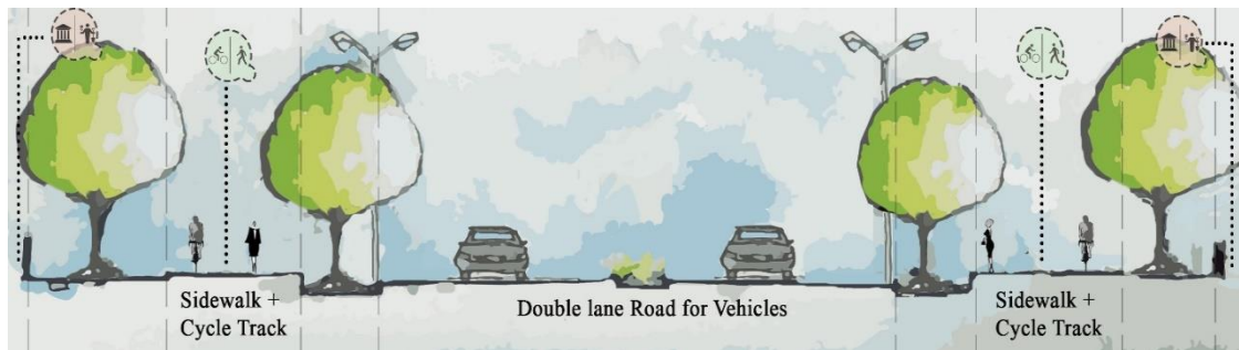
Figure 4: The section of V2 and V3 streets; (hand sketched by the main author)
