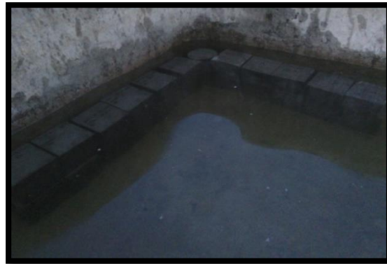
Curing of Specimens
