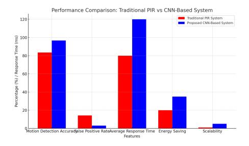
System Performance Comparison (Traditional PIR vs Proposed CNN): This chart compares the two systems across various features such as Motion Detection Accuracy, False Positive Rate, Average Response Time, Energy Saving, and Scalability. The CNN-based system outperforms the traditional PIR system in terms
