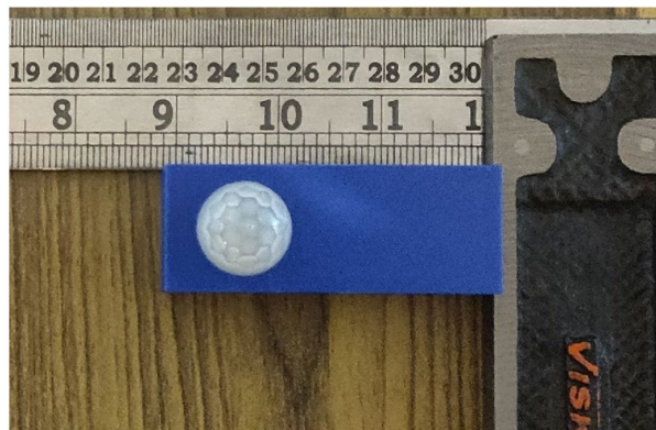
Figure 4 Size of the Device 80 x 40 x 25 mm (L x W x H)
