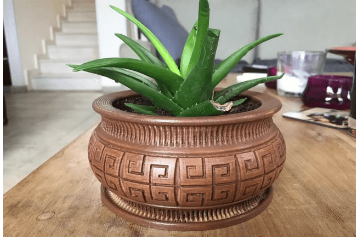
Figure 22 A 3D Printed Wood Filament Pot, The Sculpture was Sanded After the 3D Printing Process Theias (2022)
