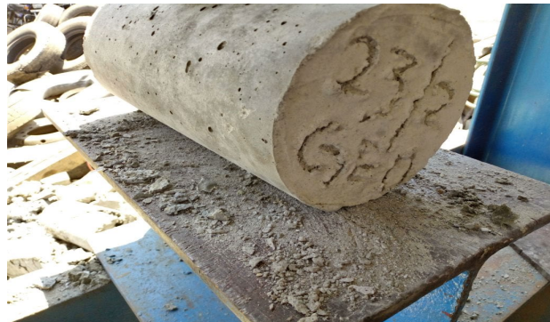
Fig 2 Split Tensile Test of Cylinder
