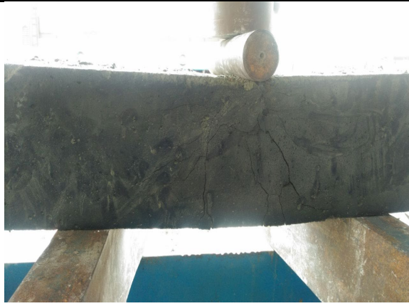
Fig 3 Flexural Strength Test Of Beam
