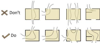
Locate inlet openings perpendicular to (or at most  $\pm 45^{\circ}$  from) the prevailing winds. Locate outlet openings on the opposite side of inlet openings, and make them equal to, or greater in size than, the inlet opening
