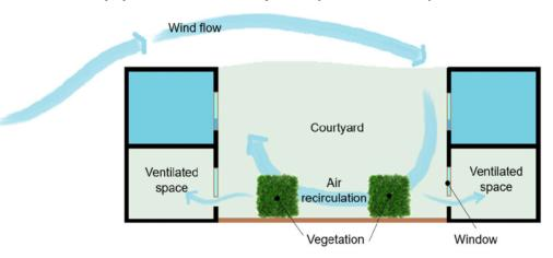
**(iv)Building Form and Massing:** The form and massing of buildings influence their aerodynamic properties and airflow patterns. Designing buildings with streamlined shapes and minimizing obstructions such as protruding elements or adjacent structures can reduce air resistance and enhance cross-ventilation effectiveness.
